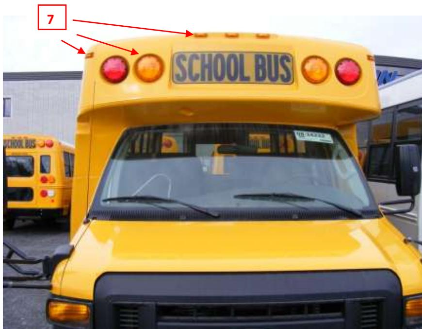
7. If everything has been well sealed and water is still infiltrating, then you might want to check the marker and warning lights. (If the vehicle has light hoods, you may add sealant to the screw holes)
