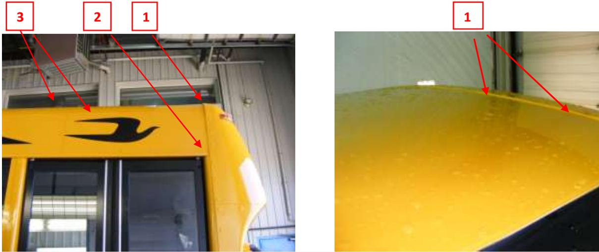
1. On top of bus, check for cracks or unsealed areas where the roof cap meets the roof skin. At the front of the bus as well as at the rear. **Because of the G5 ergonomics, it is possible that a rear leak will result in water spots in front of the vehicle.**
