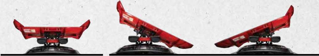
Straight-ahead scoop mode Angled right for windrowing Angled left for windrowing
