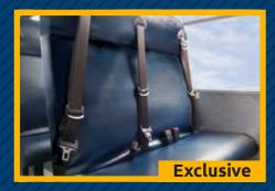
Integrated child seats and 3-point lap and shoulder seat belts are available for enhanced safety and versatility. \*FMVSS 208 requires 3-pts seat belts in all school buses with a GVWR less than 10,000 lbs.
