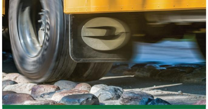
Blue Bird performs full vehicle accelerated durability testing that approximates 300,000 miles service life of the vehicle at an automotive proving ground. This rigorous evaluation includes cobblestones, inverted chatter bumps, impact bumps, undulated road, staggered bumps for chassis torsion and resonance road.
