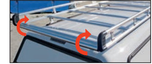
Easy-Loading Roller System Allows ergonomic loading and unloading of ladders, reducing stress and injuries. One person can easily load the ladders without damaging the vehicle.
