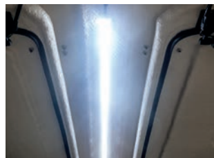
LED Rope Light Option Activated When Any Door Opens
