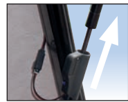
Optional Prop Switch turns your lights on/off, when you open/close your door.
