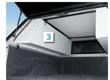
Toolboxes are securely fastened to roof framework
