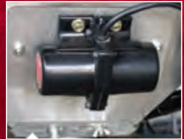
Optional vibrator helps keep material moving.
