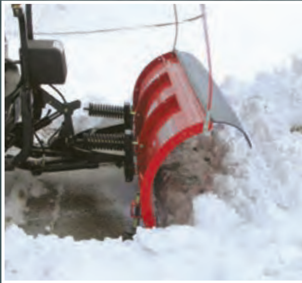
Progressive action full-trip design activates compression springs for trouble free performance.
