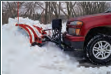
26" tall stainless steel moldboard plows and stacks with ease. Torsion trip edge provides protection on irregular surfaces.
