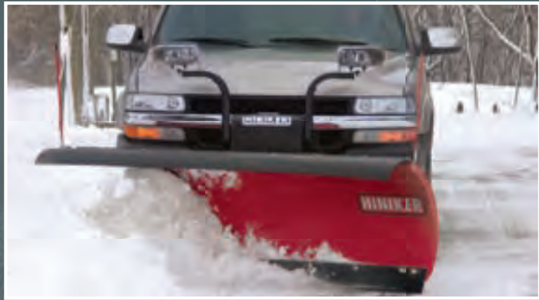
Polyethylene snow deflector (optional) provides a slick surface for smooth snow flow.
