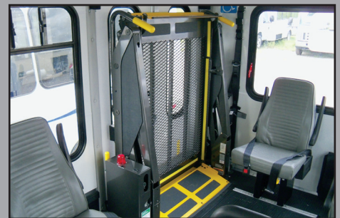
Optional ADA wheelchair lift mounted in the rear of the bus
